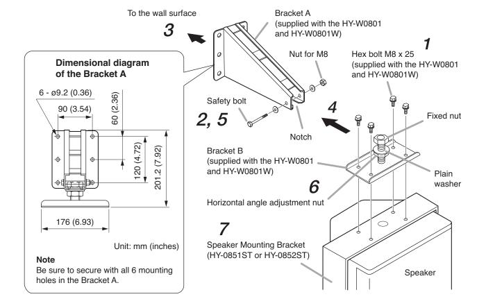
Step 1. Attach the Bracket B to the HY-0851ST or HY-0852ST Speaker Mounting Bracket.
